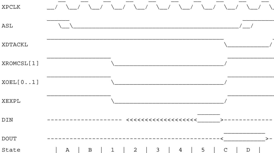
For a write cycle the write strobes have this timing
