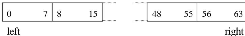
In the big-endian system, the left-most pixel is always the most significant. The left-most pixel therefore always includes bit 63. In byte address terms this is stored in byte 0.
