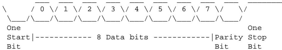
The parity can be ODD, EVEN or none. The polarity of both the output and the input can be programmed to be active high or low. The polarity shown is active low.
